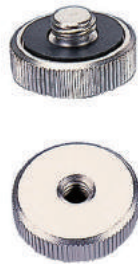
UN-5695 Retaining Screw TC/BE Size:φ25 x 8(H)mm Weight:31g Upper Screw:φ3/8" Lower Screw:φ1/4"
