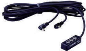
UNP-7308 Multi Synchro Tap For 2 camera /3strobe Distributor Size: 12(H)X14(W)X41(D)mm Weight:69g X-contact/terminal cord:2M flash/terminal cord 1M
